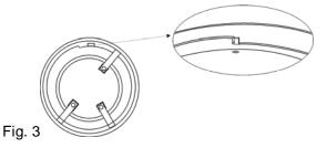
Remove tab carefully using a pair of pliers.
